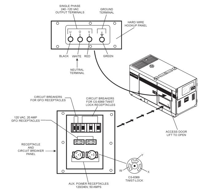
Figure 8. Output Terminal Panel
